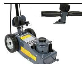
8. Replace the Filler Bung and turn the Release Valve to the raise position, depress the trigger holding down until the Lift Ram has extended to full stroke then continue to hold the trigger down for 10 seconds. Turn the Release Valve to lowering position and lower the Lift ram to lowered position.
