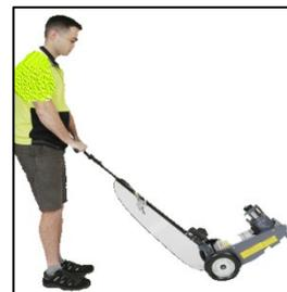
6. Lower the jack back to the floor and continue to depress the trigger mechanism until the lift ram is fully extended holding the trigger open for 10 seconds.
