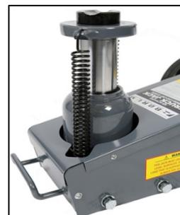
7. Turn the Release knob slowly to lower position and allow the lift ram to fully retract.
