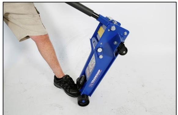
7. Place jack on the floor and recheck the oil level, Refill to 6mm below the fill port if required before replacing the filler bung as per step 1.
