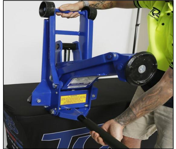
5. With the help of an assistant place jack back onto the floor and tilt on its front wheels. Rotate the release handle to the lowering position.
