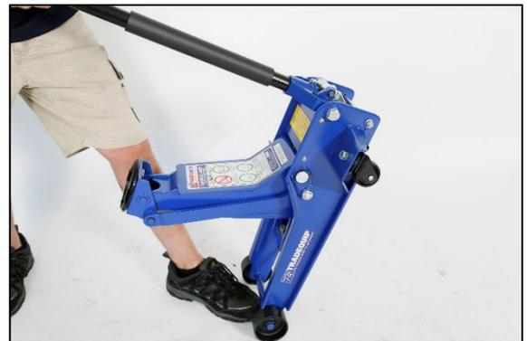
6. Ensure lift arm returns to fully lowered position
