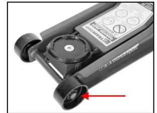
2. Wheels and Castor axles, bearing races should be lubricated with a Light Bearing Grease or 30/40W Machine Oil to ensure long life and prevent premature wear and provide smooth rotation during lift and positioning.
