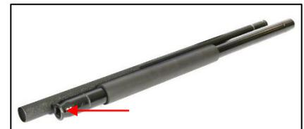
5. Lubricate the handle socket pivot bolts with 30w/40w oil to prevent premature wear of the handle socket.
