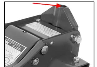
4. Lubricate with a Light Bearing grease the inner square drive in the handle spigot.
