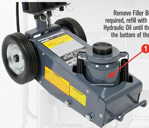
Remove Filler Bung and if required, refill with SAE 32 grade Hydraulic Oil until the oil is lapping the bottom of the filler hole.
