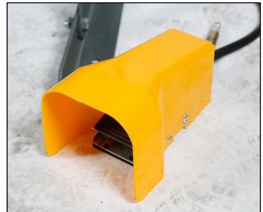
6. Turn the selector valve lever to Neutral position 2, then depress the air foot valve, keeping the air motor working no less than two minutes (120secs).
