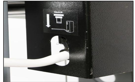
5. Connect the air supply hose to the air foot valve controller.
