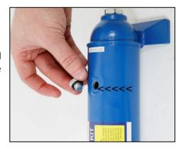
2. Disconnect the ram hydraulic coupler and remove the ram from the frame by undoing the locking collar and lifting the ram out of its headstock.
