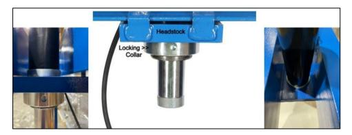
3. Lay the ram on a stand below the pump and reconnect the hydraulic supply line.
