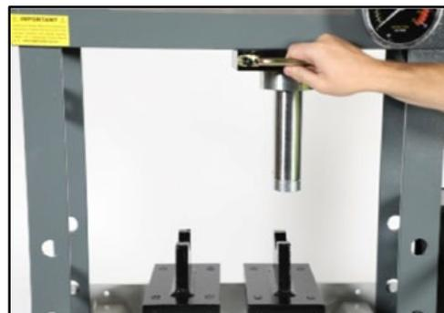
5. Open the release and allow the ram to fully retract.
