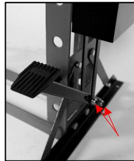
2. Bed load bearing surfaces should be lubricated with a Light Bearing Grease or 30/40W Machine Oil to ensure long life and prevent premature wear.
