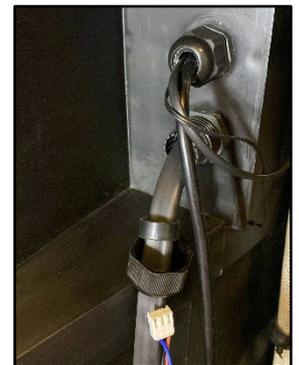
9. Feed the pump cable plug through the bulkhead fitting leaving approximately 200mm of cable on the circuit board side. Ensure the thread cable and cable braid back together.
