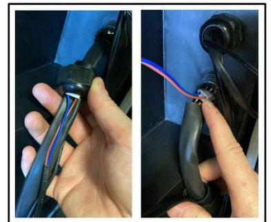
10. Connect the pump cable plug to the control panel then loop the extra cable and cable tie it, tucking this behind the control panel. Refit the control panel with the screws. Ensure the thread cable and cable braid back together.
