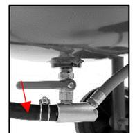
You may need to adjust a further 1/8th if a quicker cutting degree is required but keep in mind that adding media into the air stream will slow the velocity and effectiveness of the blast stream and raising the air pressure a further 10psi may be required.
