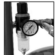
Ideal pressure will be dependent on the ability of the air supply to remain constant and without pressure drop at the gauge, as there are many variables including media type and nozzle size. However, in most cases this pressure generally around 90 to 110 PSI. Keep note that the blaster will have a peak operating pressure rating and should not be operated above this rating.
