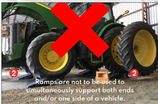
**3** Off centre loading can cause the ramp to tilt and cause possible equipment damage and or personal injury.
