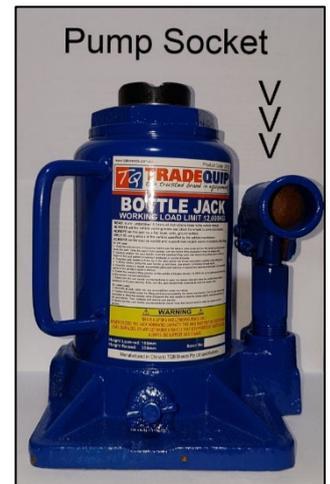
3. Turn the release valve clockwise to the lifting position.
