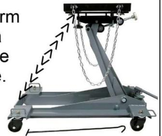
2. Remove the ram shaft retainer pin from the lift linkage
