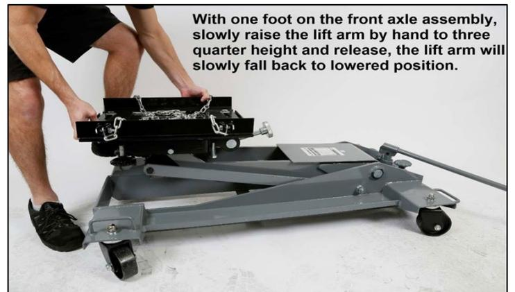
4. Remove the oil filler bung from the top of the hydraulic ram and turn the release valve anticlockwise to open.
