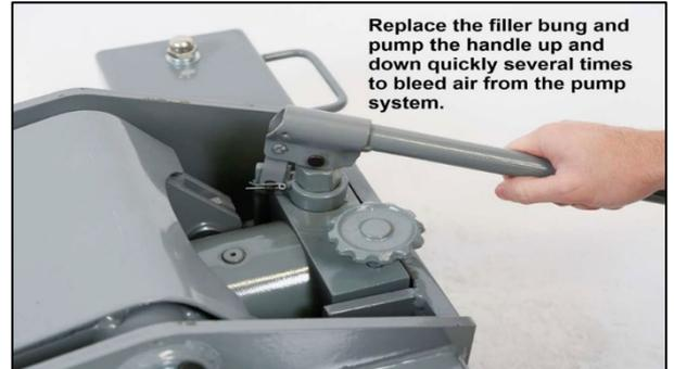
6. Recheck the hydraulic oil level and refill to 6mm below the fill port if required before replacing the filler bung.
