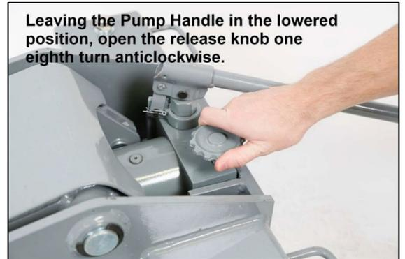
3. With one foot on the front axle assembly, slowly raise the lift arm by hand to three quarter height and release, the lift arm will slowly fall back to lowered position.
