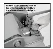
At this point both the Pump and Lift Ram should be free of air and the Jack ready for operation.
