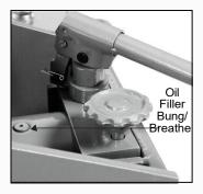
Leaving the Pump Handle in the lowered position, open the release knob one eighth turn anticlockwise.
