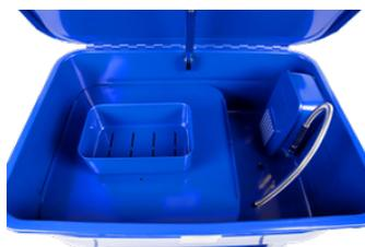
*\*Warning: For use with aqueous (water) based solutions only. Petroleum based cleaning fluids are harmful and will damage the pump and void the warranty.*
