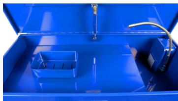
\*Warning: For use with aqueous (water) based solutions only. Petroleum based cleaning fluids are harmful and will damage the pump and void the warranty.
