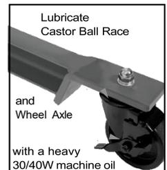
Cradle Pins, Pivots and Threaded Adjustor Rods [marked X] should be lubricated with a Light Bearing Grease or 30/40W Machine Oil to ensure long life and prevent premature wear.
