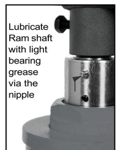
**Important:** Dirt is the greatest single cause of failure in hydraulic units. Keep the transmission lifter clean and well lubricated to prevent foreign matter from entering the system. If the Transmission Lifter has been exposed to rain, snow, sand, or grit it must be cleaned before it is stored or used.
