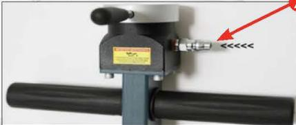
*Air motors require a minimum of 20ml of a suitable lubricant such as SAE 32 Grade Hydraulic Oil or Air Tool Lubricant at weekly intervals dependant on usage where daily/constant use may require lubrication more frequently. Please apply directly into the air trigger mechanism air supply coupling.*
