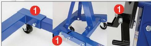
**2** Regularly lubricate all castors and wheels for ease of movement once loaded.
