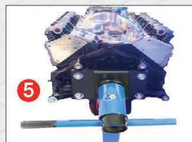
**6** Lock mounting plate in position before attaching the engine, and ensure the load is centred and securely mounted on the locking plate prior to releasing from the engine lift.
