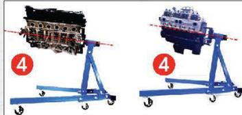
**5** Where possible minimise the extended length of the upper two attachment adaptors to reduce possible flexing of the headstock plate.
